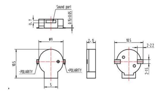
\*Unit: mm; Tolerance:  $\pm 0.3$ mm Except Specified
