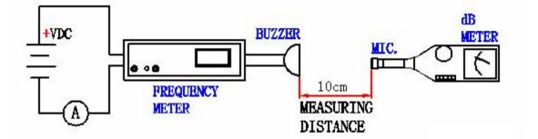
In the measuring test, buzzer is placed as follows:
