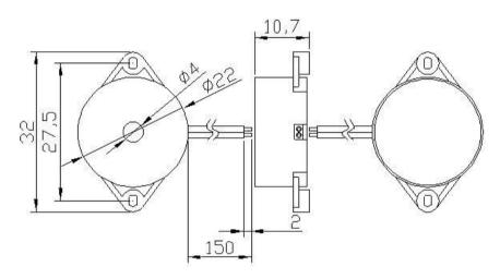
(UNIT:MM) Tolerance: ±0.2mm
